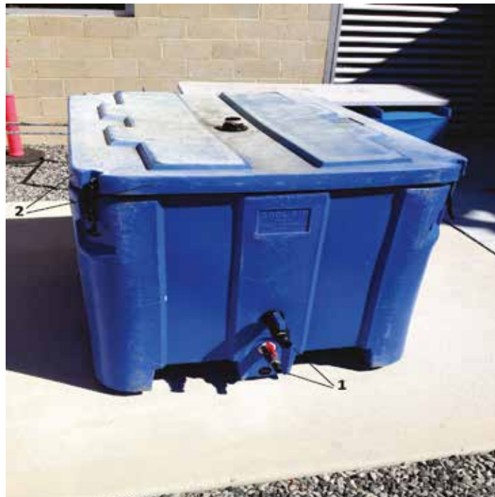
Figure 5. Esky profile during transport (1) dump valves (2) lid arrangement. 1.2.1. Esky aeration & monitoring
