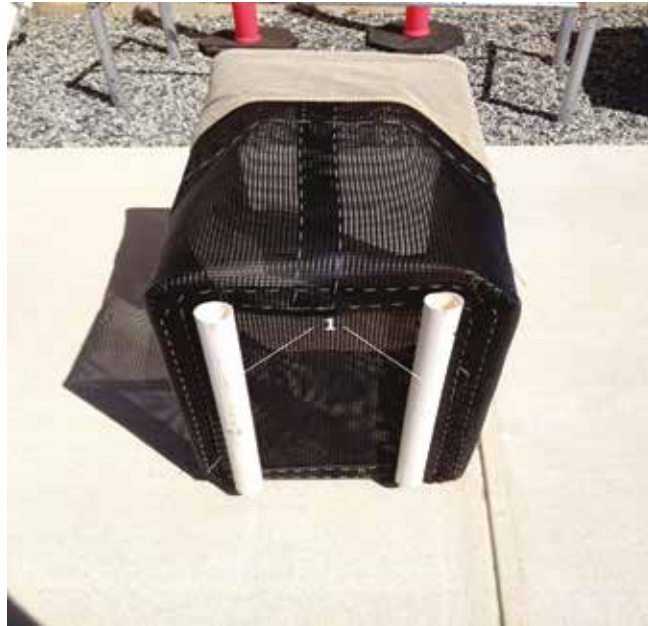
Figure 4. Basket profile. (1) Positioning of the 40 mm PVC pipe lengths.
