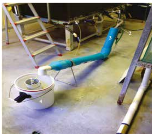
Figure 49. INVE cyst separator set-up to harvest hatched cysts: cone dump valve (1) filtered freshwater hose (2) INVE cyst separator (3) 100 \mu m harvest bucket (4)
