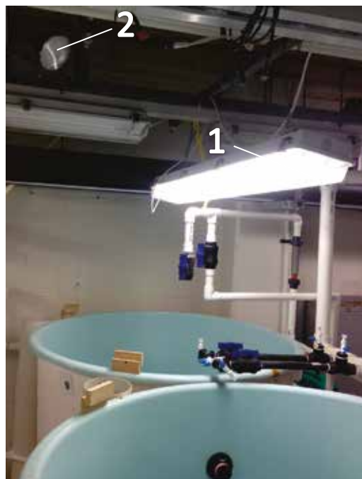
Figure 46. Fluorescent light suspended above tank (1) and 'ramp up' spotlight (2)
