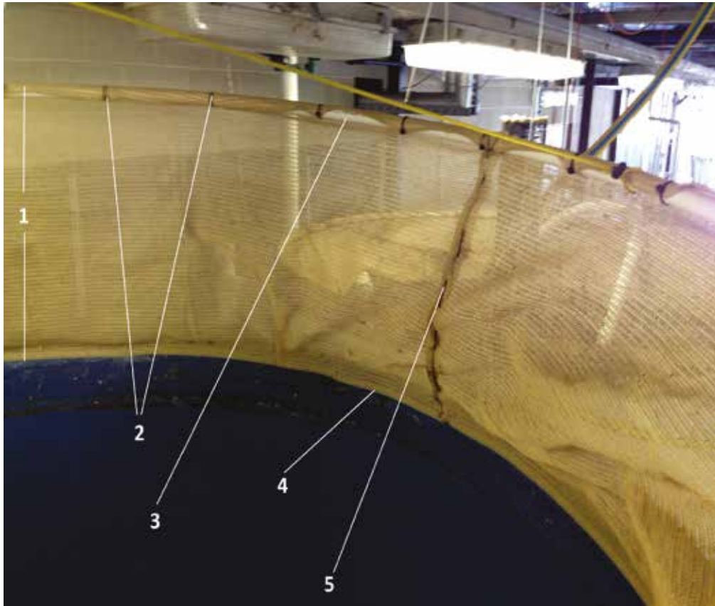
Figure 21. Shade cloth profile. (1) 500 mm height when erected (2) cable ties to attach shade cloth to the frame (3) 15 mm PVC frame (4) location of shade cloth attachment on tank (5) both ends of the shade cloth sewn together.
