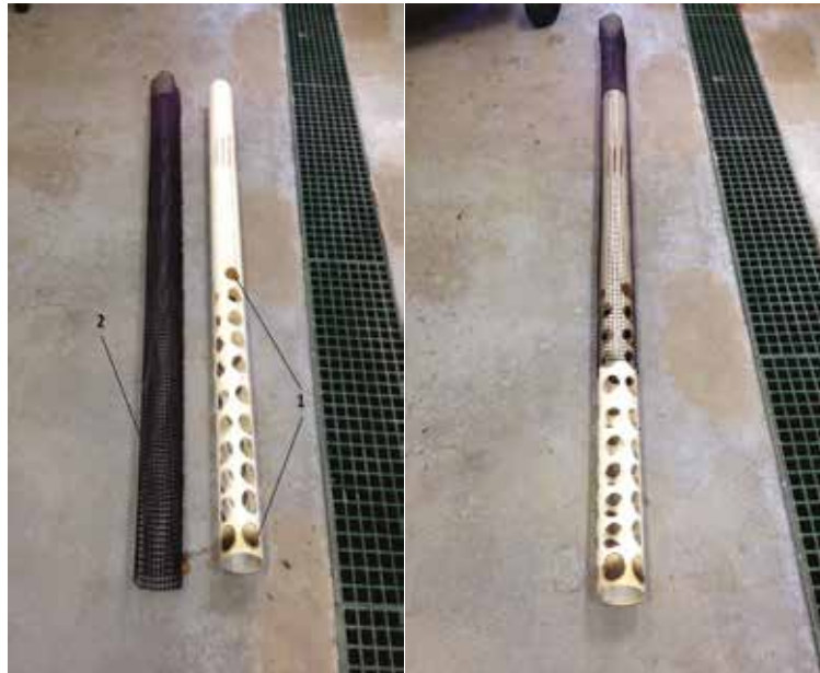
Figure 24. (1) PVC standpipe and the location of the 30 mm holes (2) oyster mesh sleeve.
