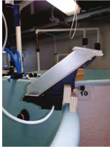
Figure 45. AMD feeder attached to tank wall
