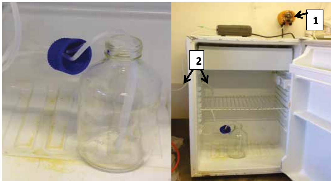
Figure 53. 2:00 am enrichment bottle connected to a peristaltic pump (1) and a feeding line (2)
