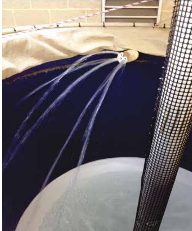
Figure 17. Incoming water in the 2000 Lt tank.
