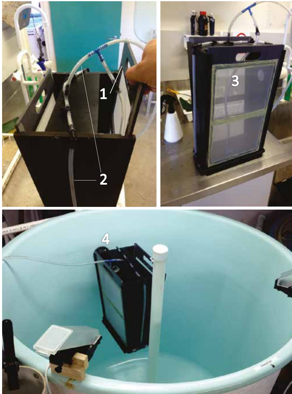
Figure 38. Interchangeable screens (1) fitted with 6 mm airline for internal and external aeration (2) Side profile of filter showing 250 \mu m mesh (3) positioning of filter inside tank (4)
