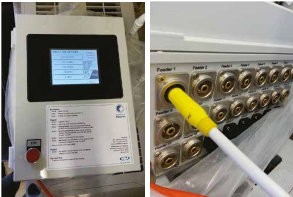
Figure 44. Front view of control box showing LCD display screen (left) and side view of cable (right)
