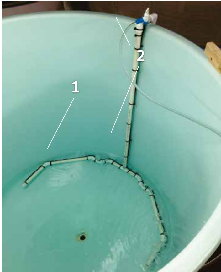
Figure 41. Aeration device showing PVC 20 mm frame (1) with 4 mm porous pipe attached (2)
