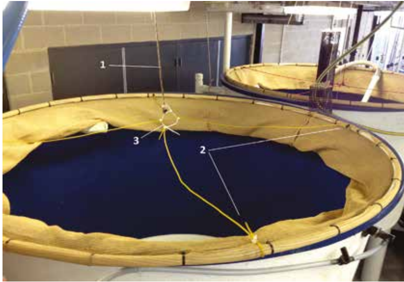
Figure 22. Shade cloth profile (1) lever attached to circular cable tie or steel ring (2) even spacing between 4 pieces of rope connected to PVC frame (3) location of circular cable tie arrangement.
