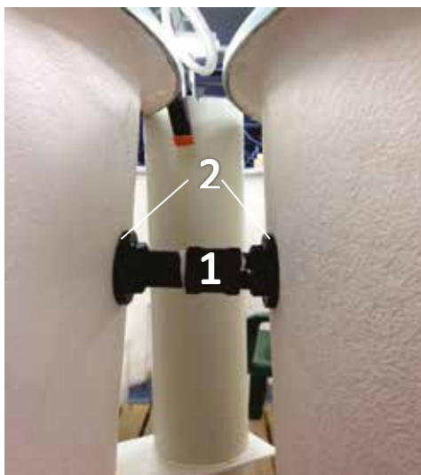
Figure 57. Two larvae tanks connected using 40 mm tank adaptors (1) and a 40 mm threaded joiner (2)
