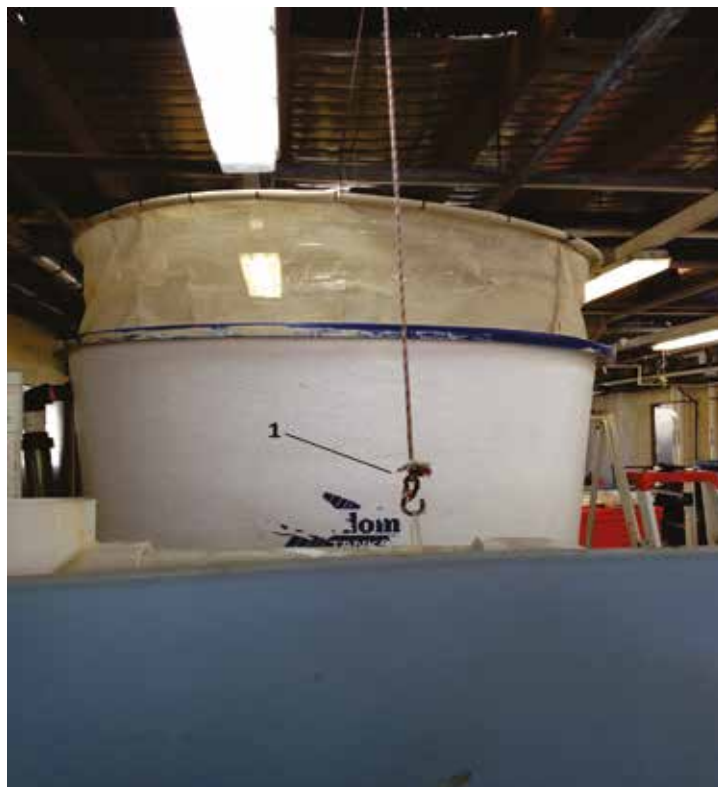
Figure 23. (1) Clip attached to the end of the lever connected to an anchor point.
