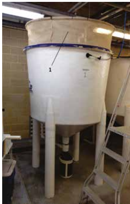
Figure 20. (1) Erected, collapsible shade cloth ring.
