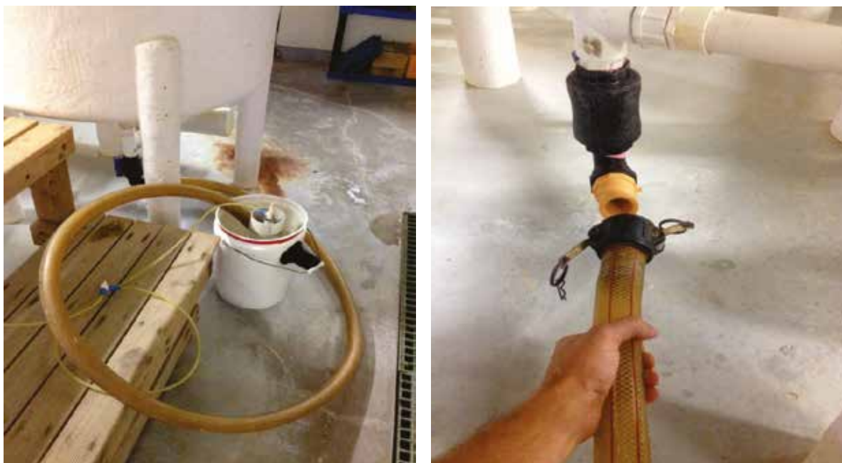
Figure 50. Harvest method of grow-out Artemia tanks (Left) Hose attachment to tank set-up (Right)
