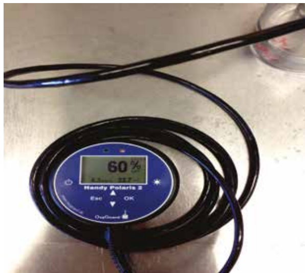
Figure 6. An Oxyguard meter reading 60% saturation (4.3 mg l -1 )
