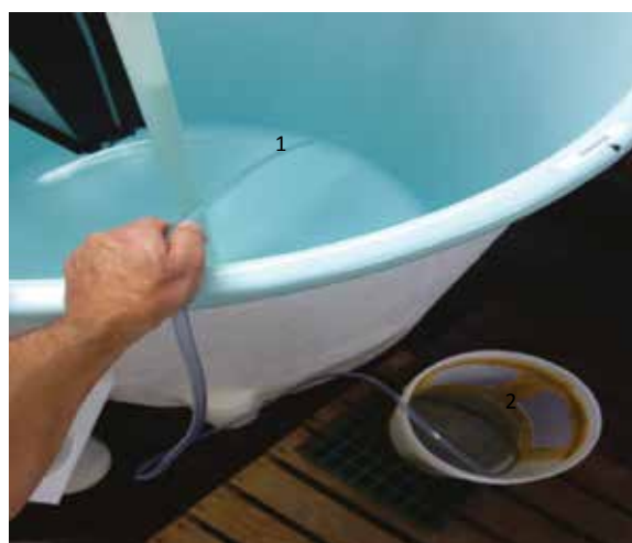
Figure 60. Siphoning method (1) acrylic rod used as the siphon tube (2) siphon hose placed in a 250 \mu\text{m} screen bucket
