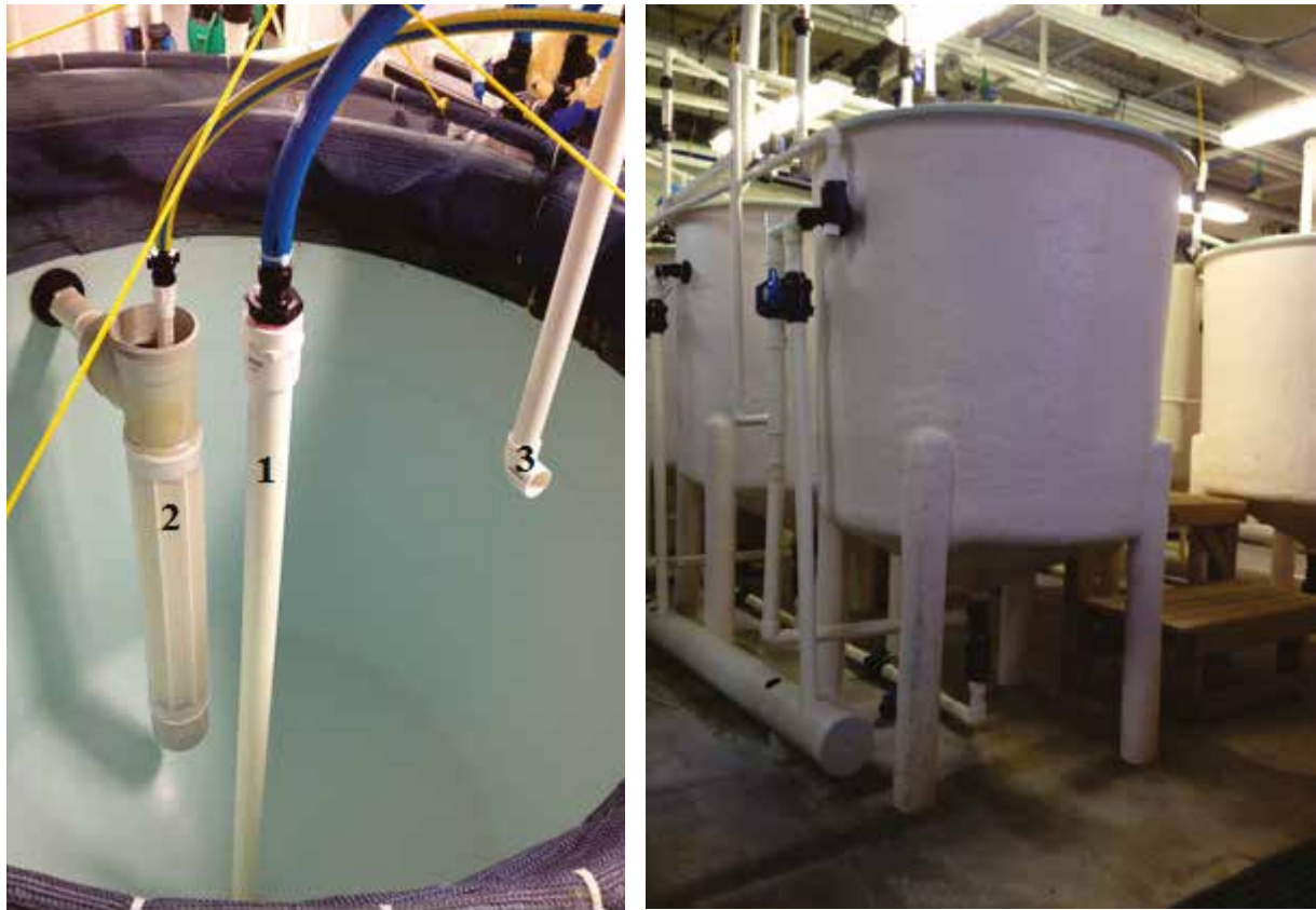
Figure 37. Artemia grow-out tank (left), (1) internal central standpipe (2) 100 µm screen filter (3) seawater inlet, Artemia grow-out tank profile (right)
