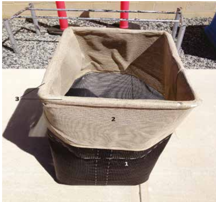
Figure 2. Basket profile (1) 5 mm oyster mesh (2) shade cloth covering (3) PVC frame at the top.
