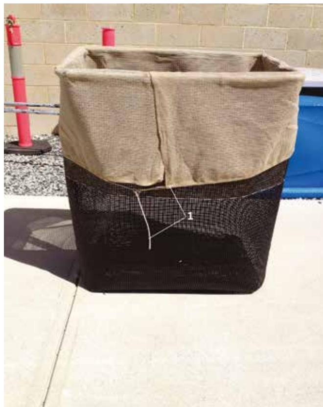
Figure 3. Basket profile. (1) Loop in exterior shade cloth and rope/elastic drawstring
