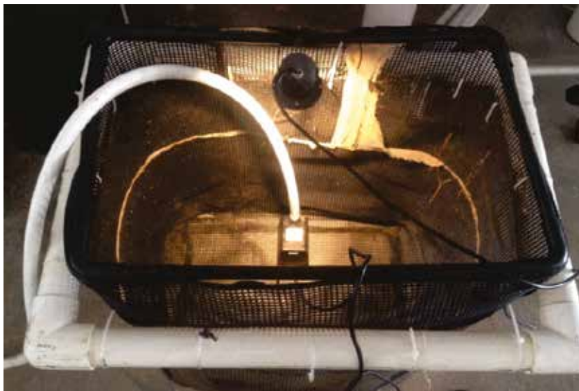
Figure 56. Plankton collector containing the submersible and pond light directly above.
